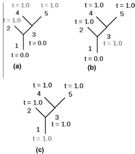
**Fig. 4.** An example of how to integrate a system. All links start at time  $t_0 = 0.0$ . (a) All leaves can be integrated, for example, to time  $s = 1.0$ . (b) Each parent of link 3 has been integrated, so link 3 can now be integrated to time  $s = 1.0$ . (c) Link 1 can now be integrated out to time  $s = 1.0$ .
