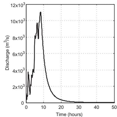
**Fig. 12.** Simulated discharge at the outlet of the Cedar River basin over two days using only channel discharge in the model. Initial channel discharge is taken as  $30.0 \text{ m}^3/\text{s}$  at each link.
