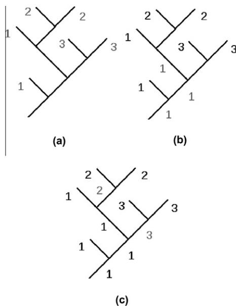
**Fig. 8.** An example of how to partition the system amongst three processes. Labels on the links represent process assignment: (a) first assign the leaves from left to right (the results of a depth-first search), (b) assign the links to process 1 starting from the leaves assigned to process 1, (c) repeat for the leaves assigned to processes 2 and 3.
