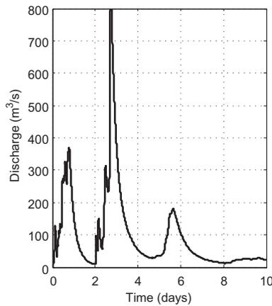
**Fig. 10.** Simulated discharge at the outlet of the Cedar River basin over 10 days for the comparison with DOPRI5. An initial discharge of  $1.0 \text{ m}^3/\text{s}$  and no initial hillslope ponding applied at each link.
