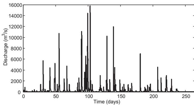
**Fig. 14.** Simulated discharge at the outlet of the Cedar River basin with radar-derived rainfall forcing using the channel discharge with hillslope model.
