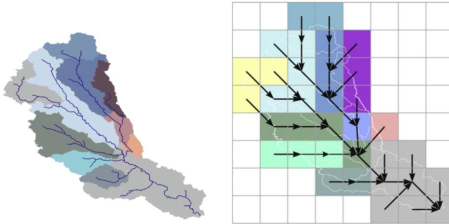
**Fig. 1.** Partitioning schemes in distributed hydrological models that lead to a global system of ODEs. Sub-watershed partitioning on the left and square pixel partitioning on the right.
