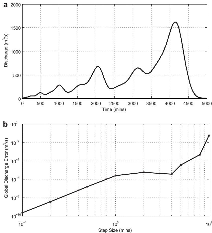
**Fig. 9.** Exact solution and numerical error for the simulated discharge of the Peano network of Horton order 10.
