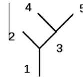
Fig. 3. Tree representation for the explicit example. The edge labeled 1 corresponds to the system  $\frac{dy_1}{dt} = f_1(t, y_1, y_2, y_3)$ , the edge labeled 2 corresponds to the system  $\frac{dy_2}{dt} = f_2(t, y_2)$ , etc. The vertices of the tree have been suppressed. The edges are directed down.
