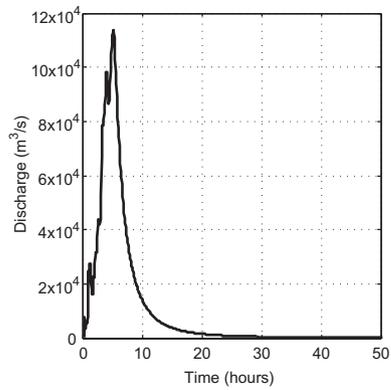
**Fig. 13.** Simulated discharge at the outlet of the Cedar River basin over two days with no rainfall forcing using the channel discharge with hillslope model. Initial channel discharge is taken as  $30.0 \text{ m}^3/\text{s}$  and an initial ponding depth is taken as  $0.1 \text{ m}$  at each link.
