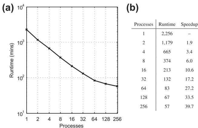
**Fig. 15.** Runtimes for the river basin model with precipitation using the channel discharge with hillslope model. Runtimes are given in minutes.
