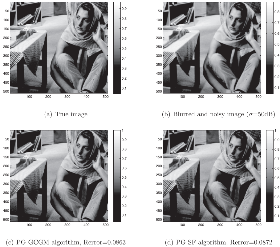
Figure 11. True image and its blurred and noisy observation together with reconstructions x^* for \eta = 0.7 .
